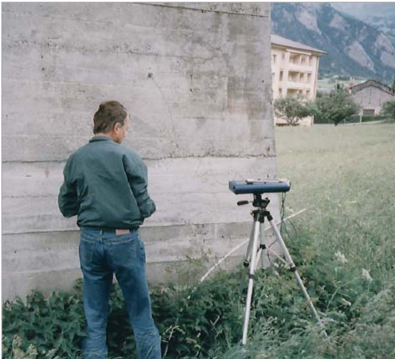
Fig. 4 und 5: Measurement of the structure-borne sound velocity level at the bridge column
